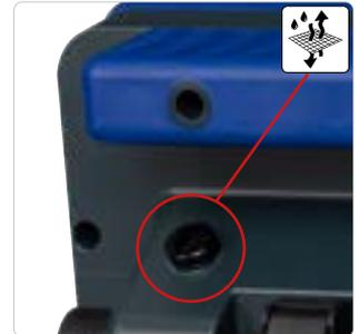
It is not enough to simply seal the luminaire as hermetically as possible to protect the electrical components from moisture and dirt. Especially outdoors, pressure builds up in the sealed housing due to changing temperatures and environmental influences. On the one hand, this leads to the formation of condensation and, on the other hand, damages the seal so that moisture and impurities can penetrate.
