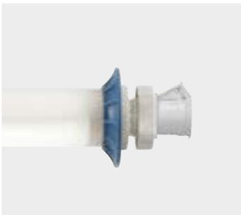
Protection tube made of impact-resistant opal plastic (polycarbonate), plastic end caps (grey/ polyamide), control gear and battery integrated, 2 protectors (blue), 5 m supply cable with mains plug, emergency light function with reduced luminaire luminous flux for 60 min, emergency function for transport / storage can be switched off, 3 emergency light cycles á 60 min. possible with full battery.
