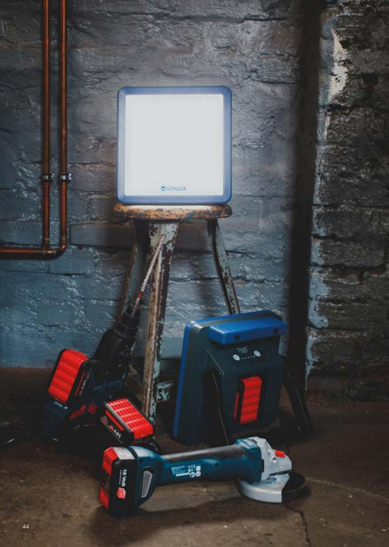
Housing plastic anthracite/blue (polycarbonate, edge protection with soft thermoplastic elastomer - TPE), cover plastic opal (polycarbonate), handle plastic black (ABS), 5-stage switchable, with light level indicator.
