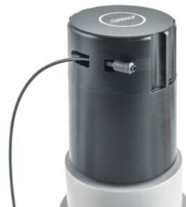
Special housing on caps for lacing. Lacing through special high-resistance cable made up of seven stainless strands, and covered by anti-scratch teflon black tubing.
